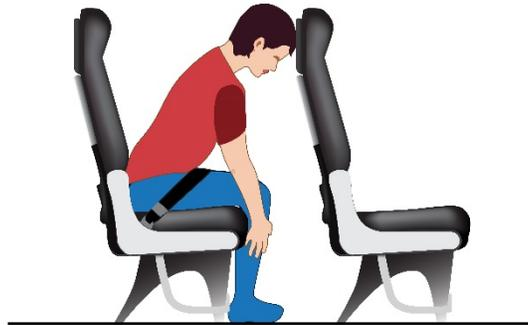
**2) Forward-Facing Passengers Seats With a Shoulder Belt.** Several air carriers have installed oblique seats (over an 18-degree angle and up to a 28-degree angle from the aircraft centerline) in their premium class cabins. Passengers should sit upright, place their chins on their sternums, their hands in their laps, and their feet flat on the floor with their knees bent at about 90 degrees, as shown in Figure 3-127.
